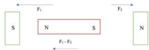
Fig.2 Unstable equilibrium phase of mechanism—Free body Diagram
