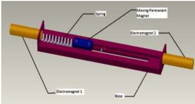
Fig.3 The construction of the reciprocating mechanism.
