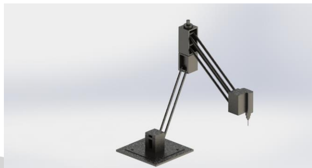
Fig. 2 Assembly of 360° degree flexible drilling machine
