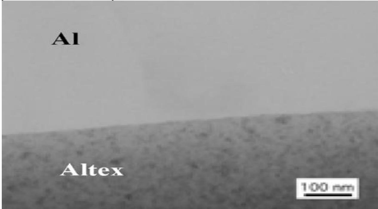
Figure 4 Formation of bonding and interface between aluminum matrix and reinforcement by addition of magnesium
