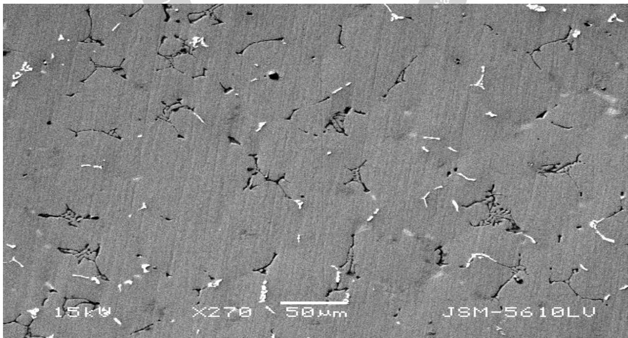
Figure 3 Scanning Electron Micrograph of Al – Mg (MnO<sub>2</sub>) composite at 270 X magnification
