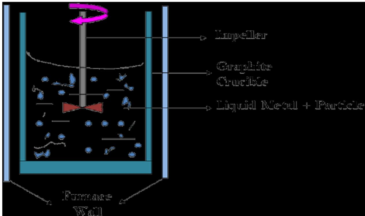
Figure 1 Line diagram of stir casting
