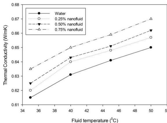
Figure 4.6: Variation in thermal Conductivity (W/mK) of Al<sub>2</sub>O<sub>3</sub>/water nanofluid recorded as a function of fluid temperature (°C).
