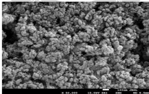
Figure 3.1: Image of dry and agglomerated Al<sub>2</sub>O<sub>3</sub> nanoparticles (Image courtesy: US research nanomaterials, Inc).
