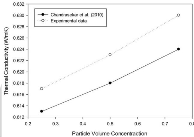
Figure 4.5: Variation in thermal Conductivity (W/mK) of Al<sub>2</sub>O<sub>3</sub>/water nanofluid recorded as a function of particle volume concentration.
