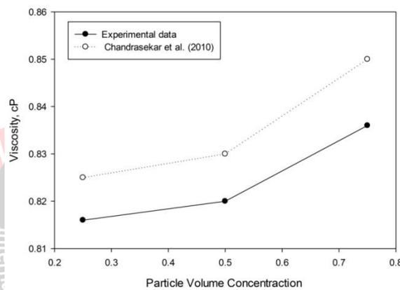
**Figure 4.7: Variations of the Viscosity of Al<sub>2</sub>O<sub>3</sub>/water nanofluids recorded as a function of particles volume concentration.**
