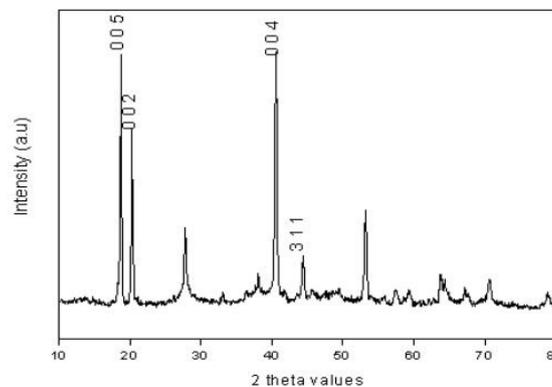
Figure 4.1: XRD patterns of  $\text{Al}_2\text{O}_3$  nanoparticles
