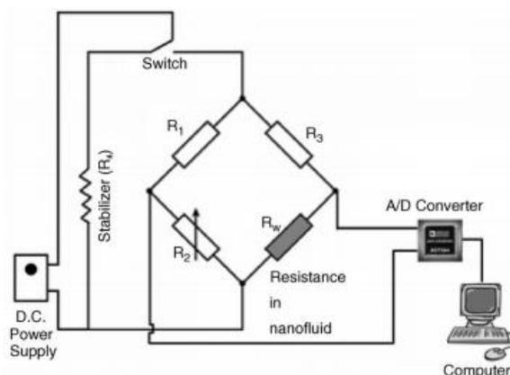
**Figure 4.4: Schematic of transient hot-wires experimental setup.**
