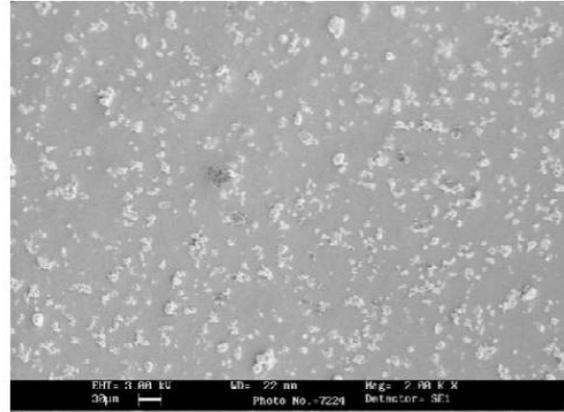
**Figure 4.3: SEM images of dispersed  $\text{Al}_2\text{O}_3$  nanoparticles in water.**
