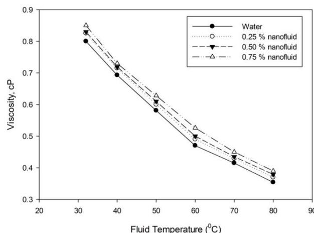
**Figure 4.8: Variations of the Viscosity of Al<sub>2</sub>O<sub>3</sub>/water nano fluids recorded as the function of nanofluid temperature.**
