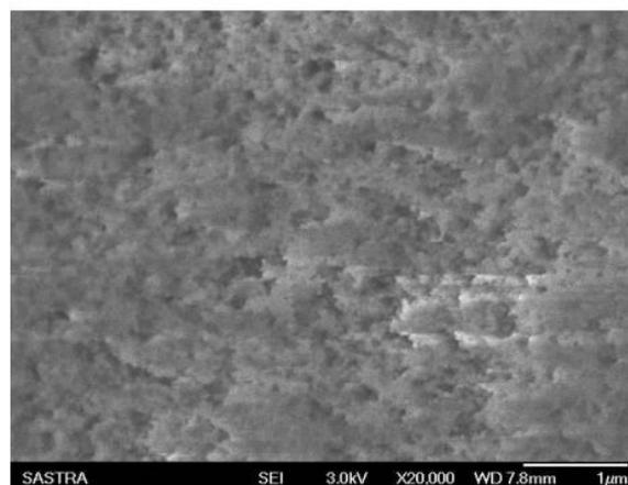
Figure 4.2: SEM images of dry  $\text{Al}_2\text{O}_3$  nanoparticles
