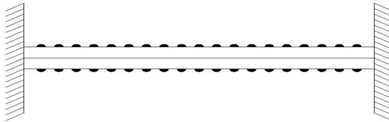
Fig: 1.2 Fixed-Fixed Condition of Riveted Joints
