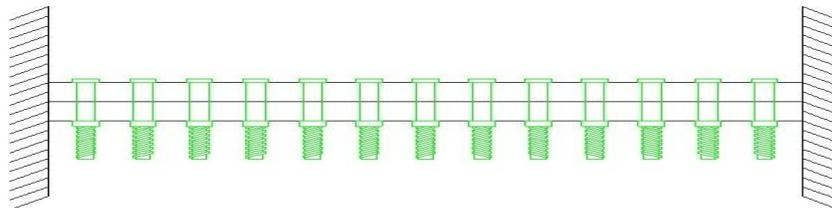
Fig: 1.4 Fixed-Fixed Condition of Bolted Joints
