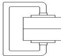
Fig: 1.8 Clamped Joint
