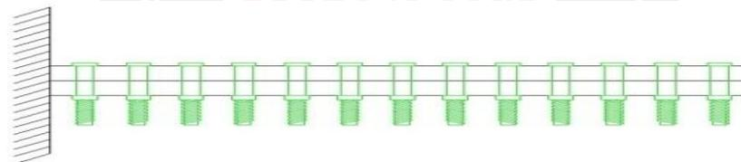
Fig: 1.5 Fixed-Free Condition of Bolted Joints
