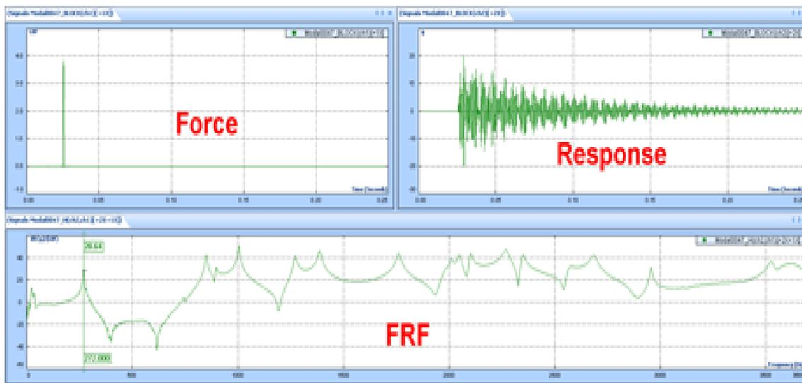
Fig: 5.4 Frequency Response Curve
