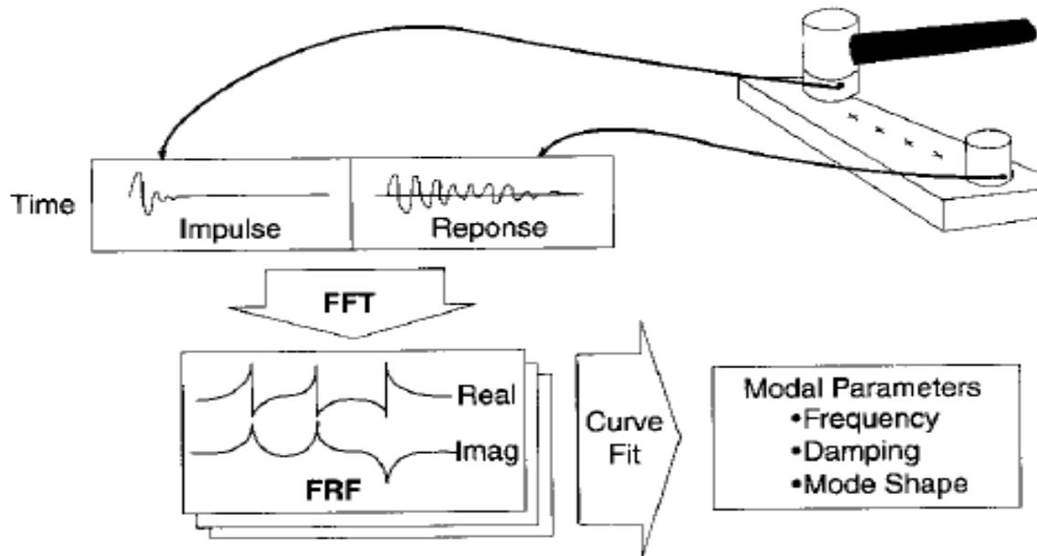
Fig: 5.2 Schematic Diagram of model testing
