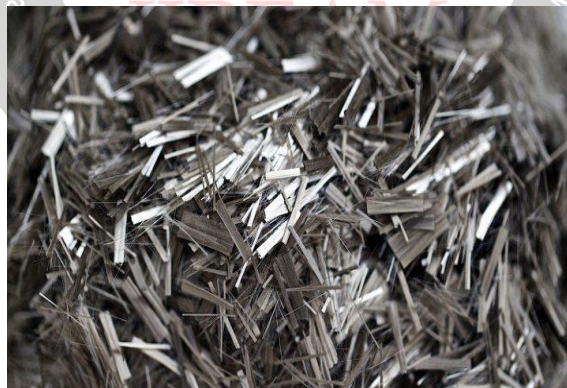
Figure2: Basalt Fiber Table 2 Properties of Basalt Fiber
