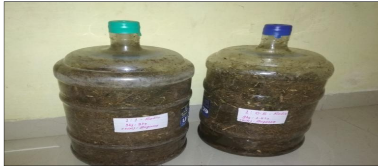
Fig. 4: Discontinuous Type Anaerobic digester with different ratio of water hyacinth and sugarcane bagasse
