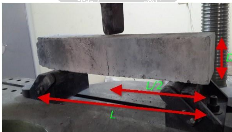
Figure.4.2: Centre Point Loading Setup In Flexural Test
