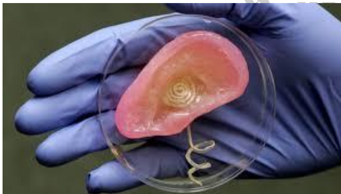
Fig: 5 final 3D printed bionic ear
