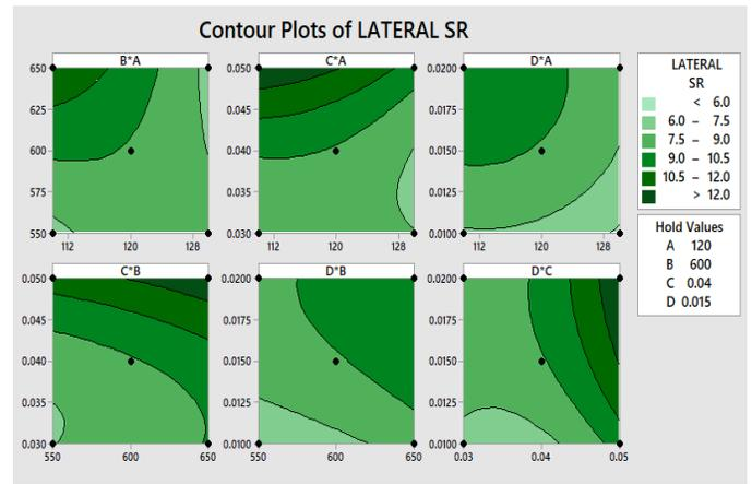
Fig. 5 Interaction contour plot lateral surface roughness Vs. Process parameters
