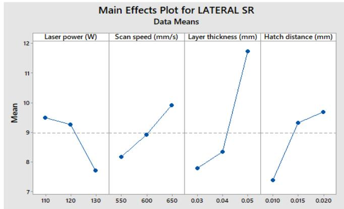
Fig. 2 main effect plot of Lateral Surface roughness
