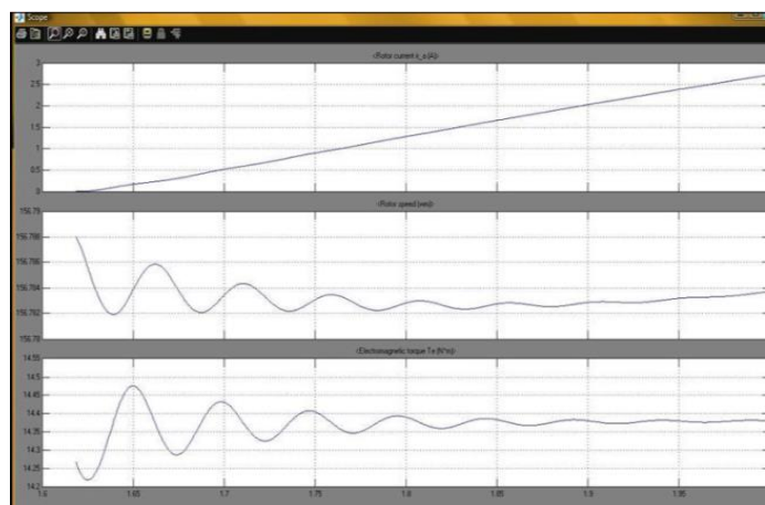
Fig: 6 OUTPUT PLOT showing O/P TORQUE and SPEED of rotor
