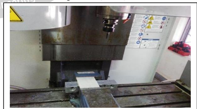
Figure 3. Machining of GFRP by CNC vertical machining center with carbide End Mill
