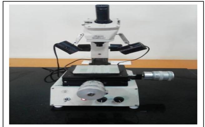
Figure 5. Measurement of of delamination damage using Tool makers Microscope
