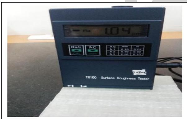
Figure 4. Measurement of surface roughness using from Surface roughness tester TR100
