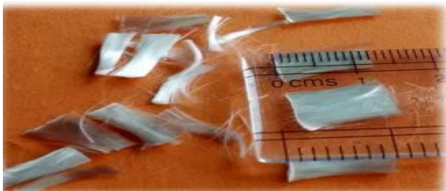
Figure:4 Polypropylene fibre showing 12 mm average size
