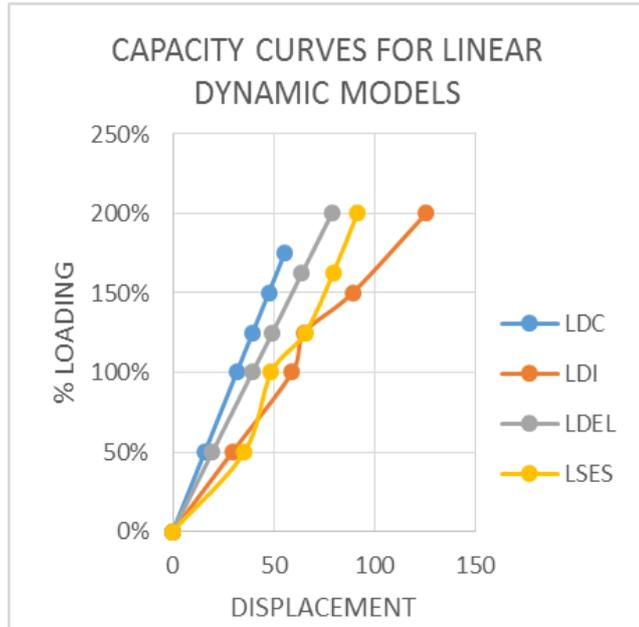
Figure 4: Combined Capacity Curves for Linear Dynamic model
