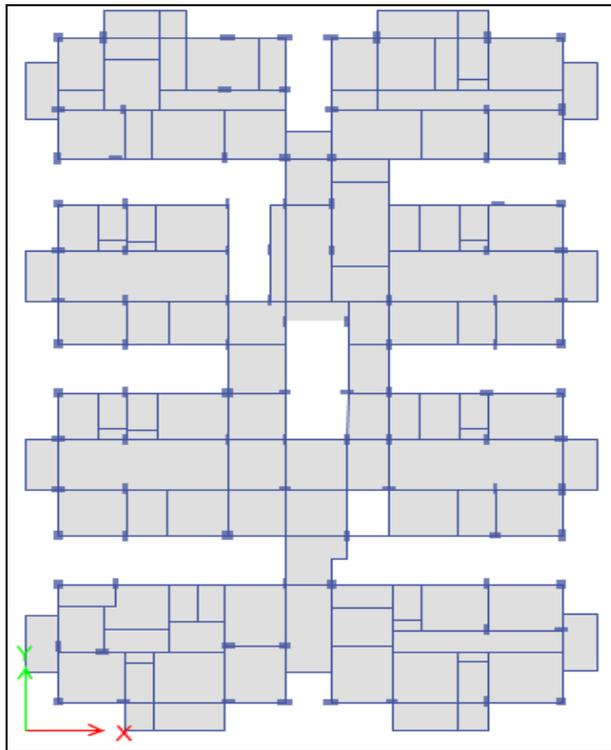
Figure 1: Plan showing beam layout of the building in ETABS
