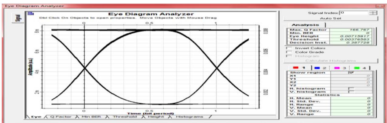
Fig.4 Output eye at the receiver end for a transmission rate of 1 Gbps
