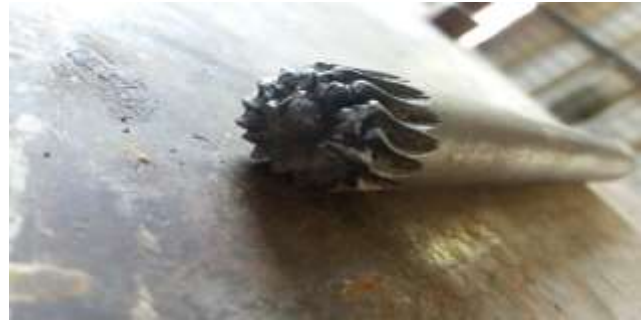
Failed drive shaft under running condition
