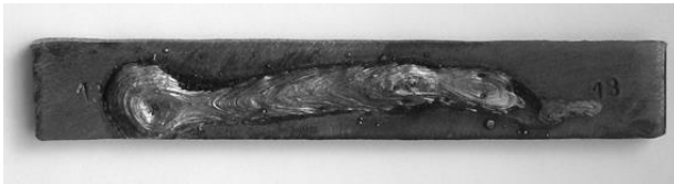
Fig. 3.3 Specimen weld beads obtained with wet welding underwater using covered electrodes
