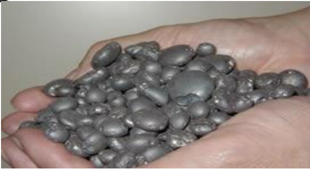
Fig.4-Iron Nuggets manufactured through ITmk3
