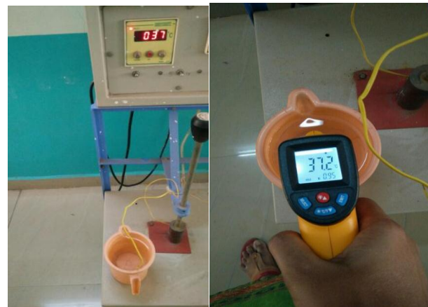
Fig.6 Comparing laser thermometer with thermocouple 2.6 Observation Table
