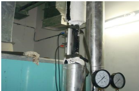
Fig.2 Water flow measurement using Ultrasonic flow meter
