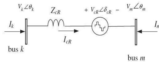
Figure 2 Equivalent circuit of SSSC
