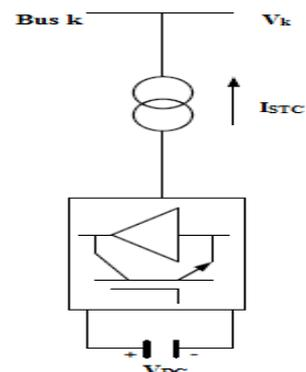
Figure 4 Equivalent circuit of STATCOM
