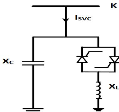
Figure 3 Firing angle model of SVC
