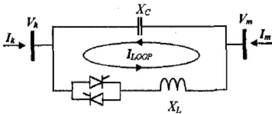
Figure 1 Equivalent circuit of TCSC
