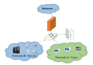
Fig 1.1Distributed Intrusion Detection System
