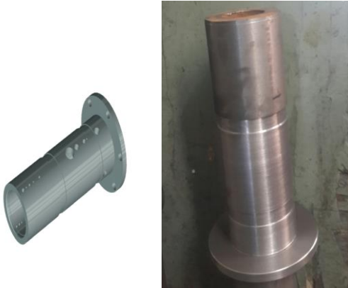
Fig. 2 - 3D Model and Actual Work piece
