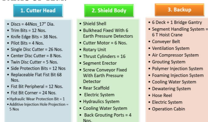
Chart 1. TBM Parts
