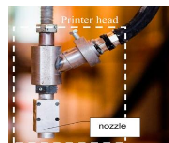
Figure 8 Printer head and nozzle
