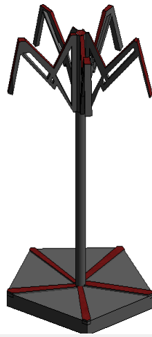
Fig 4: vertically deployed central stem along with levers deploying (shown without plates)
