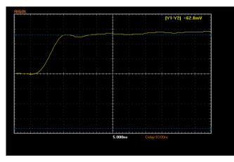
Fig. 10. Voltage of reflected waveform with 470 $\Omega$  resistor
