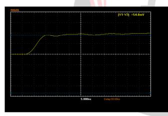
Fig. 9. Voltage of reflected waveform with 227  $\!\Omega$  resistor
