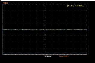
Fig. 7. Voltage of reflected waveform with 75  $\!\Omega$  resistor
