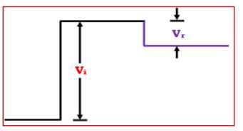
Fig. 2. Incident and Reflected waveform on TDR
