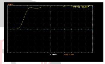
Fig. 11. Amplitude of reflected waveform with open end
