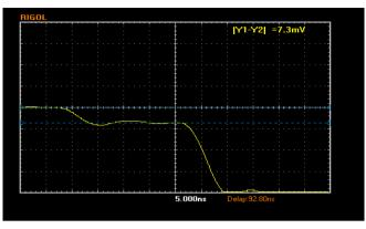
Fig. 13. Voltage of reflected waveform of  $50\Omega$  cable
