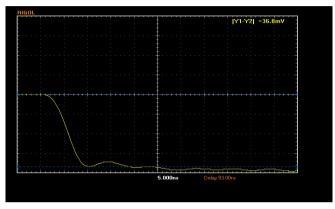
Fig. 4. Voltage of reflected waveform with short end
