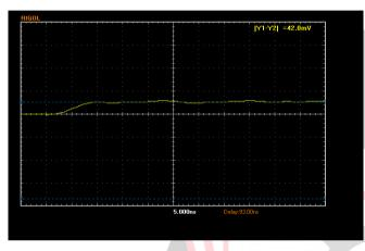
Fig. 8. Voltage of reflected waveform with 100  $\Omega$  resistor
