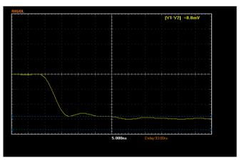
Fig. 5. Voltage of reflected waveform with  $10\Omega$  resistor
