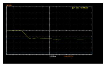
Fig. 6. Voltage of reflected waveform with  $33\Omega$  resistor
