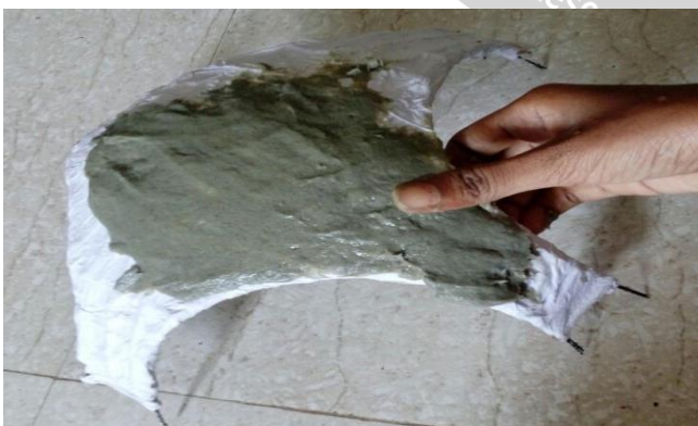
Fig 4 Applying the mixture above the mesh finish
