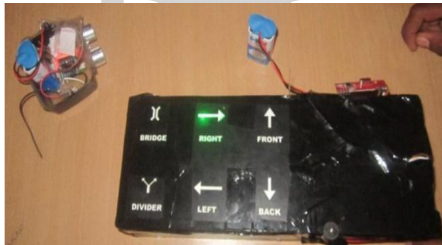
Fig 6. LED indication when suddenly vehicle coming from right side.
