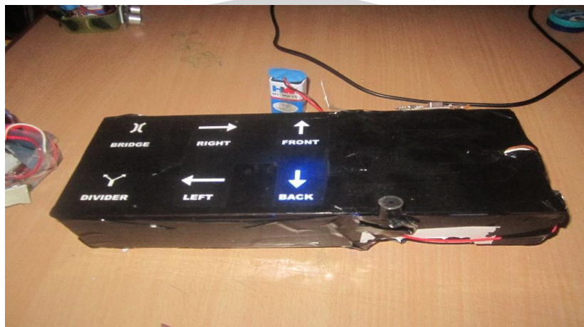
Fig 3. LED indication when suddenly vehicle coming from back side.
