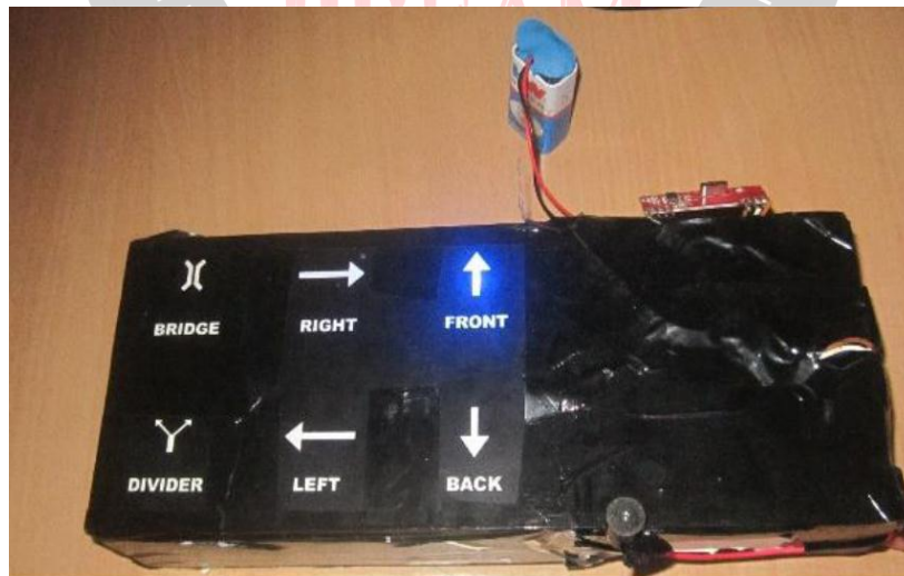
Fig. 4. LED indication when suddenly vehicle coming from front side.
