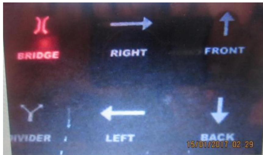
Fig 5.LED indication when there is narrow bridge at certain distance.
