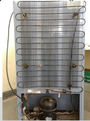
Fig 2.1: refrigerator with condenser lengths at 2.448m, 4.08m and 6.12m
