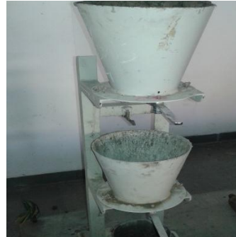
photo 2. Compaction factor test
