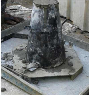
Photo 1. Slump cone test
