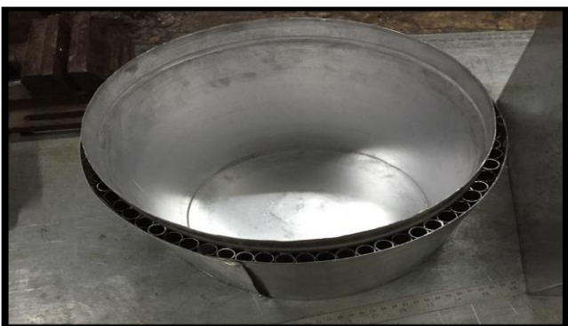
Fig. 5 Drum cover with aluminium sheet.
