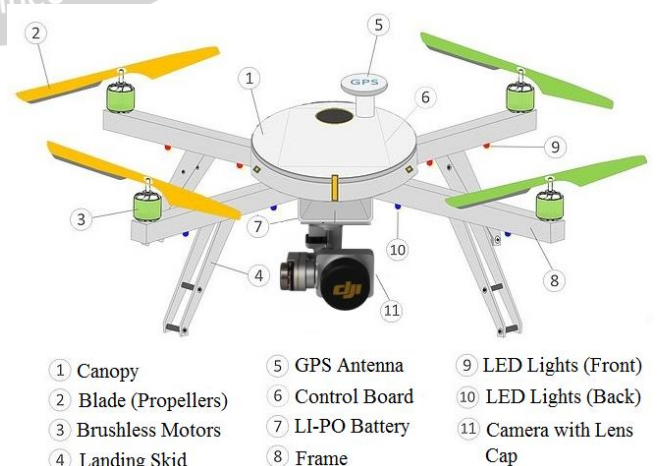
Fig. 1 Quadcopter Structure
