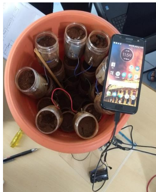
Figure 10: Charging of a Smartphone with the obtained voltage
