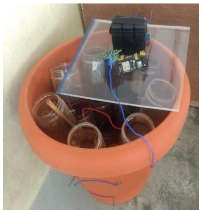
Figure 8: Cells arrangement & Circuit Setup
