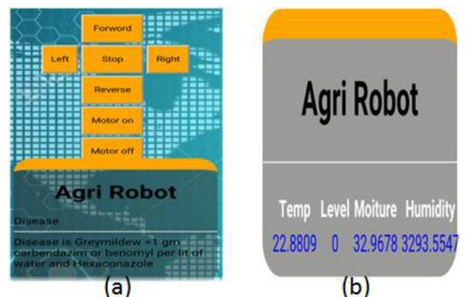
Fig. 5. (a) Android app displaying cotton leaf disease information (b) Android app displaying different sensors reading.
