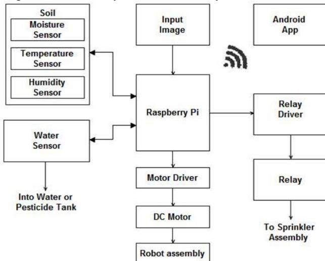
Fig. 2. Block diagram of system for cotton leaf disease detection and Remedy to it.
